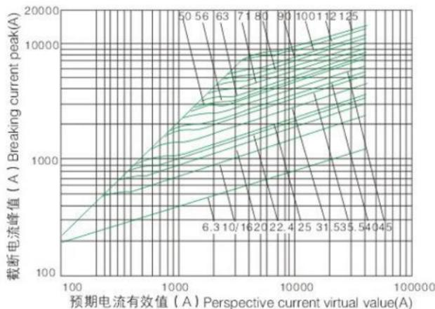
A/B型12KV熔断件截断电流特性 Breaking-current characteristics of fuse link type A/B
